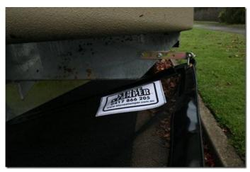
The location shown below will give better protection if the cross beam on the caravan/camper is set a long way back as the mesh goes from the width of the van to the width of the car exposing the front corners of the caravan/camper (as shown in the picture below).
