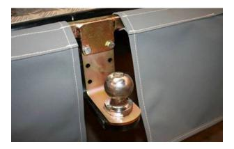
You will need a minimum of 85mm for the **Tongue option** to work well and so the coupling can turn.
